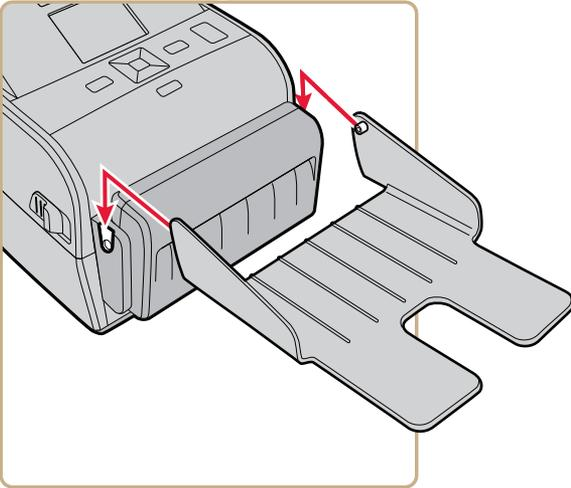
Use this tray only with the cutter accessory for the PC43d and PC43t printers.
