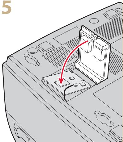
Route the antenna cable to keep clear of the access door.
