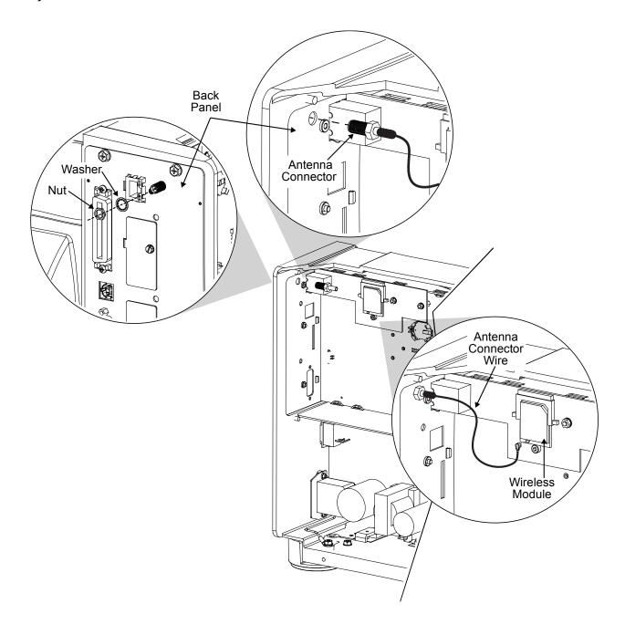
**G)** Screw the Antenna onto the Antenna Connector and pivot the Antenna up for best reception.
