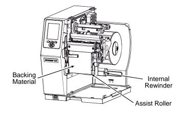
D) Wrap the Backing Material in a counterclockwise direction around the Rewinder Hub and insert the creased leading edge into one of its Slots. Insert the Media Clasp (Item ®) into the Slot over the creased leading edge of the Backing Material and around the Rewinder Hub.
