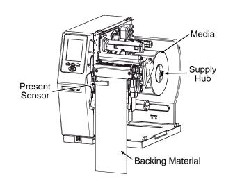
Remove the labels from this extended portion of media, leaving only the Backing Material.
