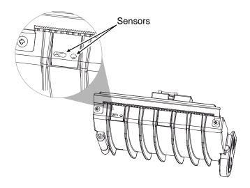
✓ **Note:** For cleaning heavy deposits, isopropyl alcohol can be used – provided it is carefully applied using a cotton swab, and then allowed to dry before reconnecting the option to the printer.
