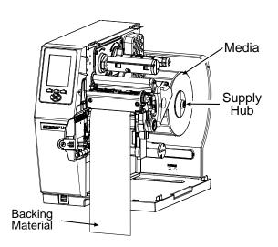
C) Route the Backing Material under the Assist Roller and the Internal Rewinder.
