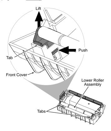
9. Take note of the individual Roller positions – they <u>must be</u> reinstalled in the same order – then, <u>carefully</u> remove the Rollers from the Lower Roller Shaft.
