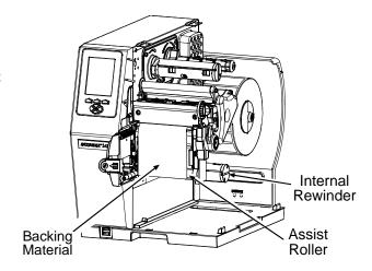
D) Wrap the Backing Material in a counterclockwise direction around the Rewinder Hub and insert the creased leading edge into one of its Slots. Insert the Media Clasp (Item ®) into the Slot over the creased leading edge of the Backing Material and around the Rewinder Hub.
