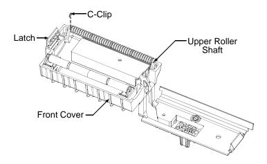
5. Remove the Upper Roller Shaft and the associated Rollers.
