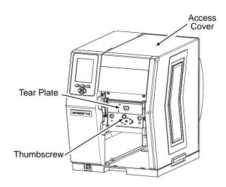
D) Remove the Thumbscrew and Tear Plate. (Alternately, if equipped with an Arc Plate, Present Sensor, or Cutter, remove that device.)
