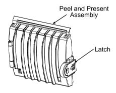
B) Carefully press the Peel and PresentAssembly into the Front Plate Connector.
