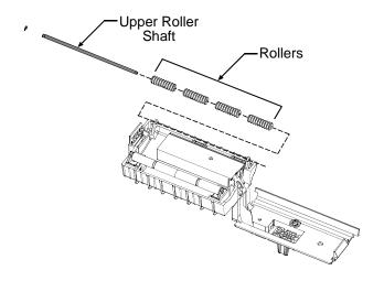
6. Using a Cotton Swab <u>dampened</u> with alcohol, wipe <u>all</u> Roller and Upper Roller Shaft surfaces clean. Pay special attention to the ridges on the Rollers to ensure that they are clean.
