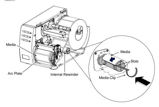
☑ Note: The Media Retainer can be used in place of the Media Clip for a more consistent rewound roll. The Media Clip and Media Retainer cannot be used together.
