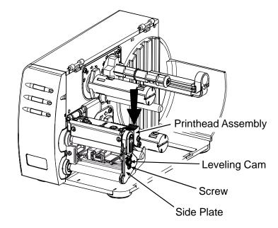
While pushing down on the Printhead Assembly, as shown, pull down on the Side Plate and tighten the Screw.
