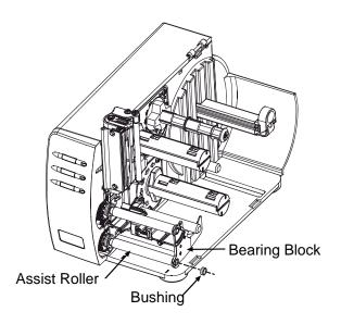
While holding the Assist Roller Bearing against the Centerplate, replace the Bearing Cap.
