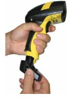
2. Insert the new battery pack containing the Magnet (included with the kit) into the reader handle. Tighten the screw to secure.
